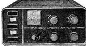
KW 1000 KW 1000 Linear Amplifier 10-80 metres. 1200 watts p.e.p. input max. Designed to be "driven" by KW 2000A/B/E or other Unit of similar power.
